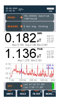
Figure 10: FFT measurement using the SMP2 + WP400.
