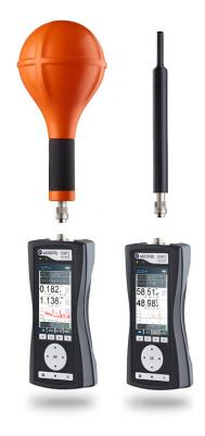
Figure 12: SMP2 EMF meter combined with the WP400 (1 Hz – 400 kHz) probe for AC magnetic field measurements (*left*) and the WPH-DC (DC – 40 kHz) probe for static magnetic field measurements (*right*).
