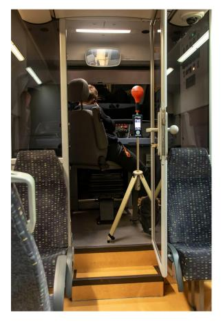
Figure 2: SMP2 + WP400 mounted on a tripod at a height of 1.5 m in the train driver cabin near the driver's seat.
