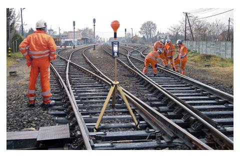
Figure 5: SMP2 mounted at 1.5 m on the center of the train track.
